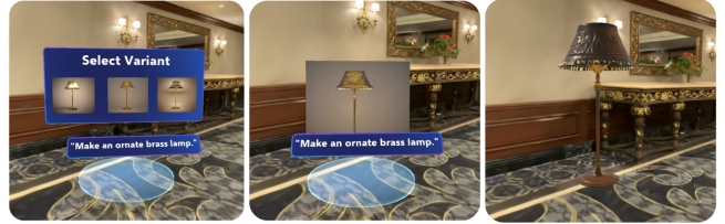
Figure 5: Object Generation via Prompting: (Left) Object generation variations from speech input. (Center) Displaying selected generation preview as a spatial annotation. (Right) Fully processed 3D generation in the scene.
