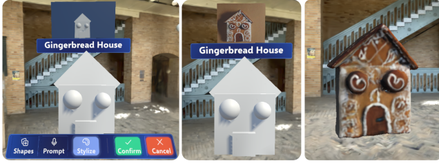
Figure 6: Object Generation via Sculpting: (Left) Sculpting toolkit to create primitive shape arrangement (Center) Displaying stylized sculpted object preview as a spatial annotation. (Right) Fully processed 3D generation in the scene.
