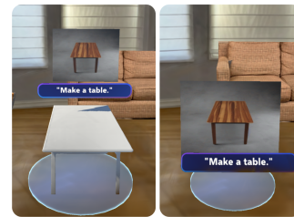
Figure 8: 3D and 2D Proxy Representations (Left) New 3D proxy showing a low fidelity mesh preview (Right) Original 2D proxy representation with image preview
