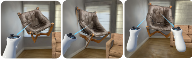
Figure 3: Object transformations and direct manipulations (Left) Positioning object in the scene (Center) Rotating object. (Right) Scaling object
