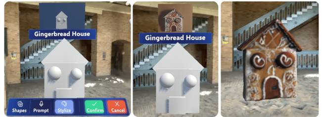
Figure 6: Object Generation via Sculpting (Left) Sculpting toolkit to create primitive shape arrangement (Center) Displaying stylized sculpted object preview as a spatial annotation. (Right) Fully processed 3D generation in the scene.
