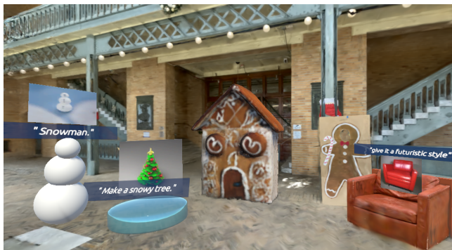
Figure 9: Spatial annotation tags are placed over the radiance field objects and generated objects with given instructions and preview generations.
